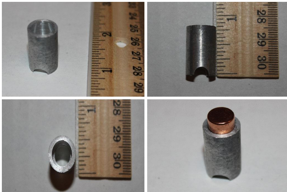
Figure 9: Aluminum Stand to Hold Hollow Point for Melting the Lead Out
