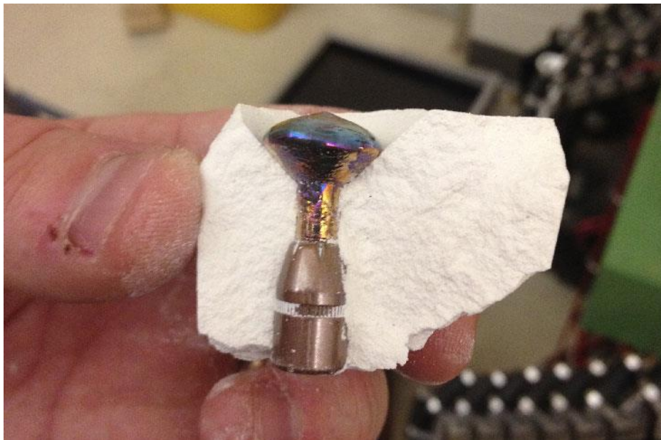
Figure 17: Split Plaster Mold Showing Freshly Cast Bismuth Bullet with “Mushroom”
