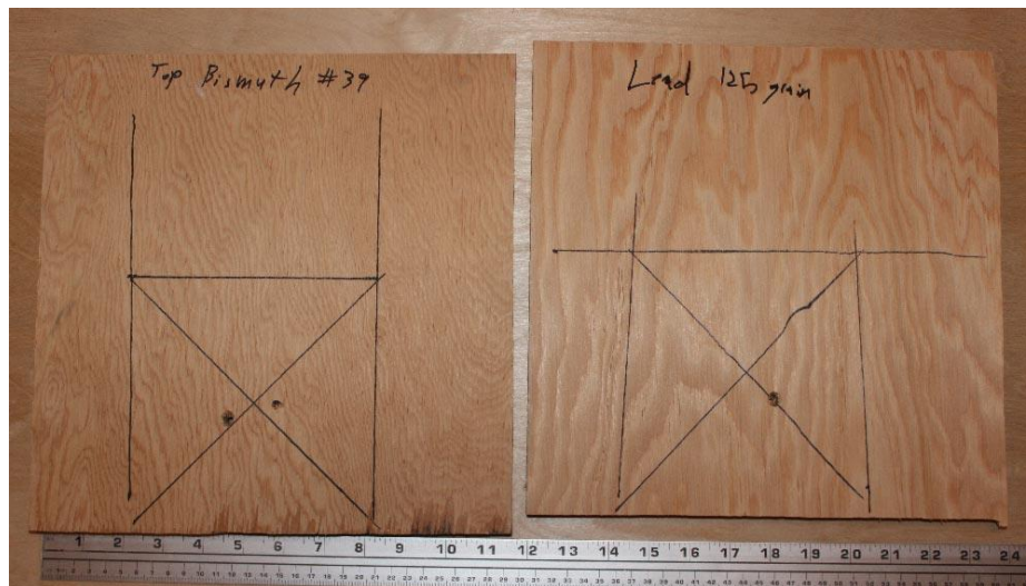
Figure 63: (Left) One Bismuth Bullet Shot through 3/4 Inch Plywood, (Right) Lead Bullet Shot into Plywood
