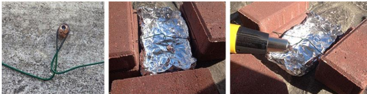
Figure 11: (Left) Bullet Held by Metal Wire, (Middle) Bullet in Place Wire Held by Bricks, (Right) Full Heating Setup
