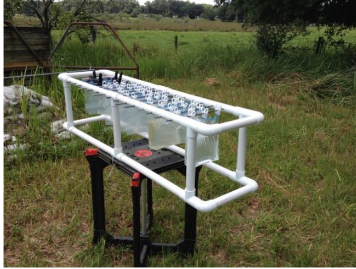
Figure 31: PVC Holding Rig Holding Water Bags
