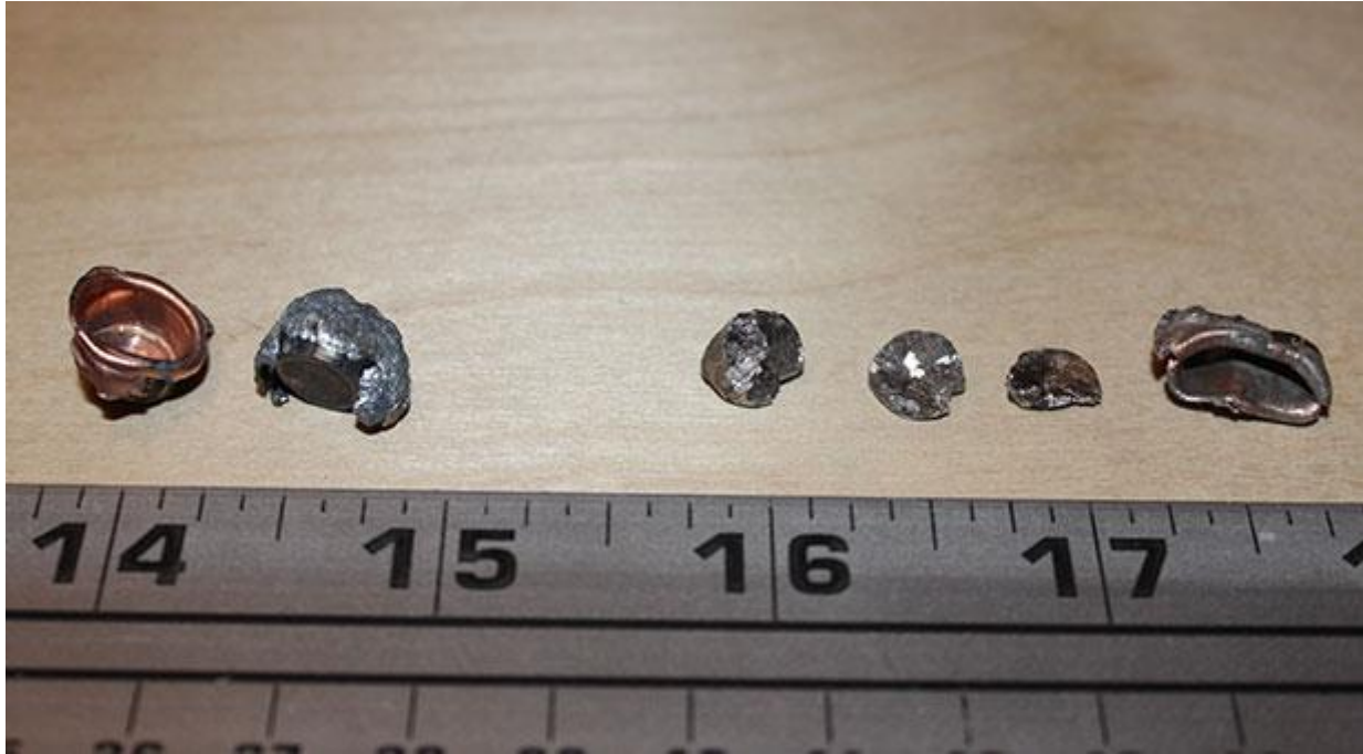
Figure 84: (Starting from the Left Going Right) Copper Jacket of Lead Bullet, Lead of the Lead Bullet, Bismuth Fragment 1, Bismuth Fragment 2, Bismuth Fragment 3, and Bismuth Copper Jacket 4
