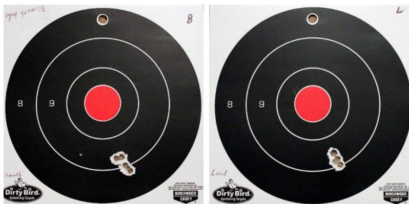
Figure 41: (Left) Four Bismuth Bullets Shot into a Target from Ten Feet, (Right) Lead Rounds Shot under Similar Conditions
