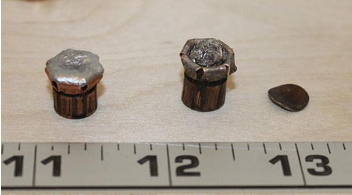
Figure 47: Bullets Shot Into Bare Gelatin, (Left) Lead Bullet, (Middle) Bismuth Bullet, (Right) Jacket Base
