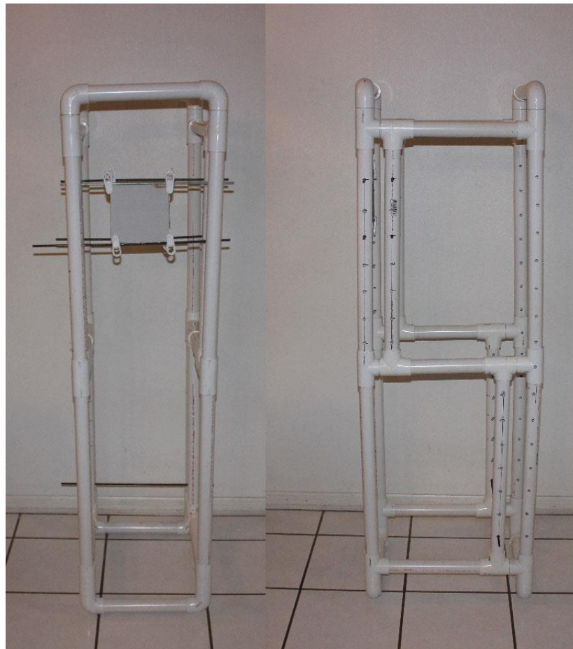
Figure 32: PVC Rig for Holding Target Materials (Left) Front View, (Right) Side View
