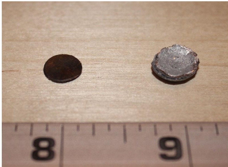
Figure 76: Fragments Pulled from the Ballistic Gelatin after Firing through Steel, (Left) Base of the Copper Jacket, (Right) Two Disks of Steel
