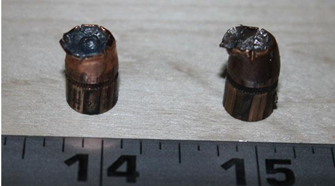
Figure 68: Side View, (Left) Lead 125 Grain Bullet Shot into Plywood, (Right) Bismuth 125 Grain Bullet
