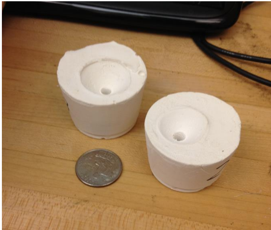
Figure 14: Plaster Mold with Jacket Entombed Inside
