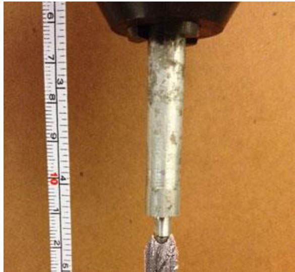
Figure 16: Hollow Point Tool Shown With Sectioned Bullet
