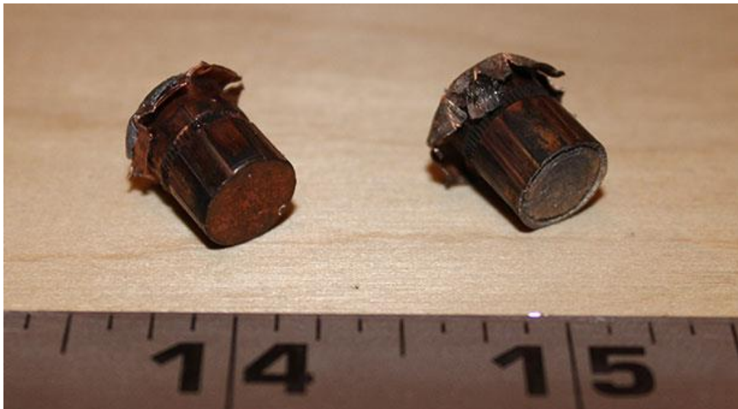
Figure 62: Base View of Bullets Shot through Gypsum Board, (Left) Lead Bullet, (Right) Bismuth Bullet
