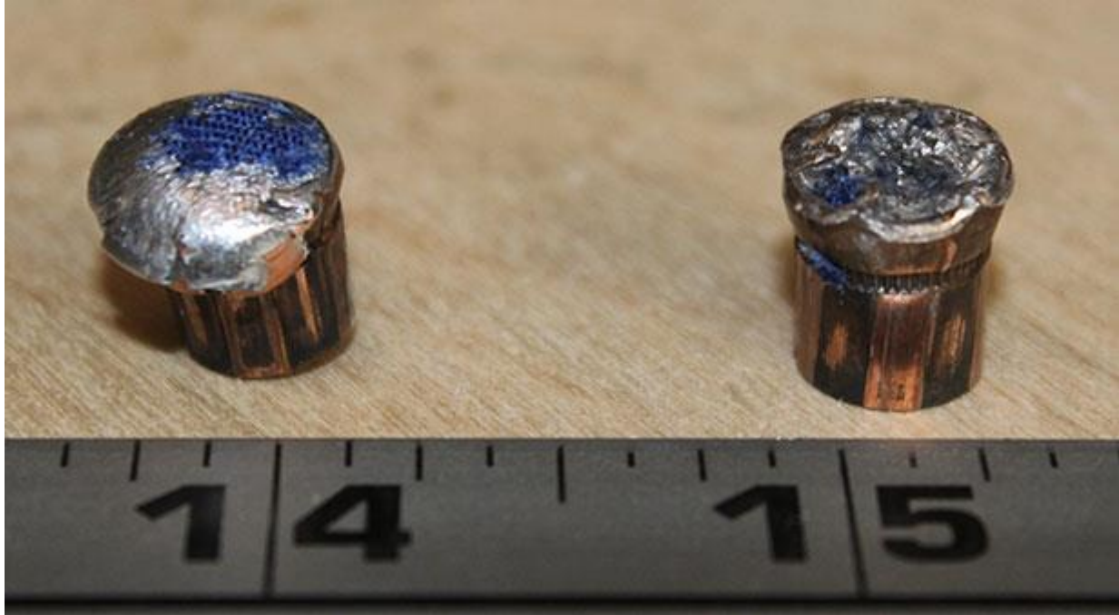
Figure 77: Bullets Shot through Steel (Left) Lead 125 Grain Bullet, (Right) Bismuth Bullet
