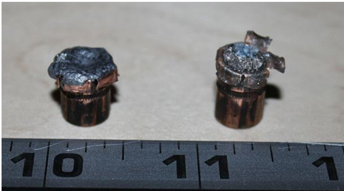
Figure 55: Bullets Extracted from Gelatin after Being Shot through Heavy Clothing, (Left) Lead Bullet, (Right) Bismuth Bullet
