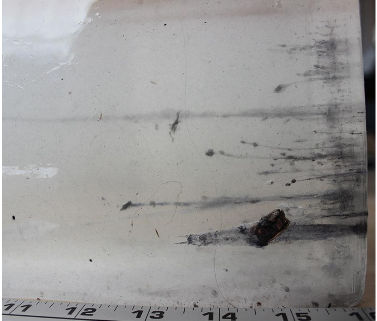
Figure 83: Bismuth Entrance Wound, Bullet Fragmented upon Going through the Auto Glass Test 1
