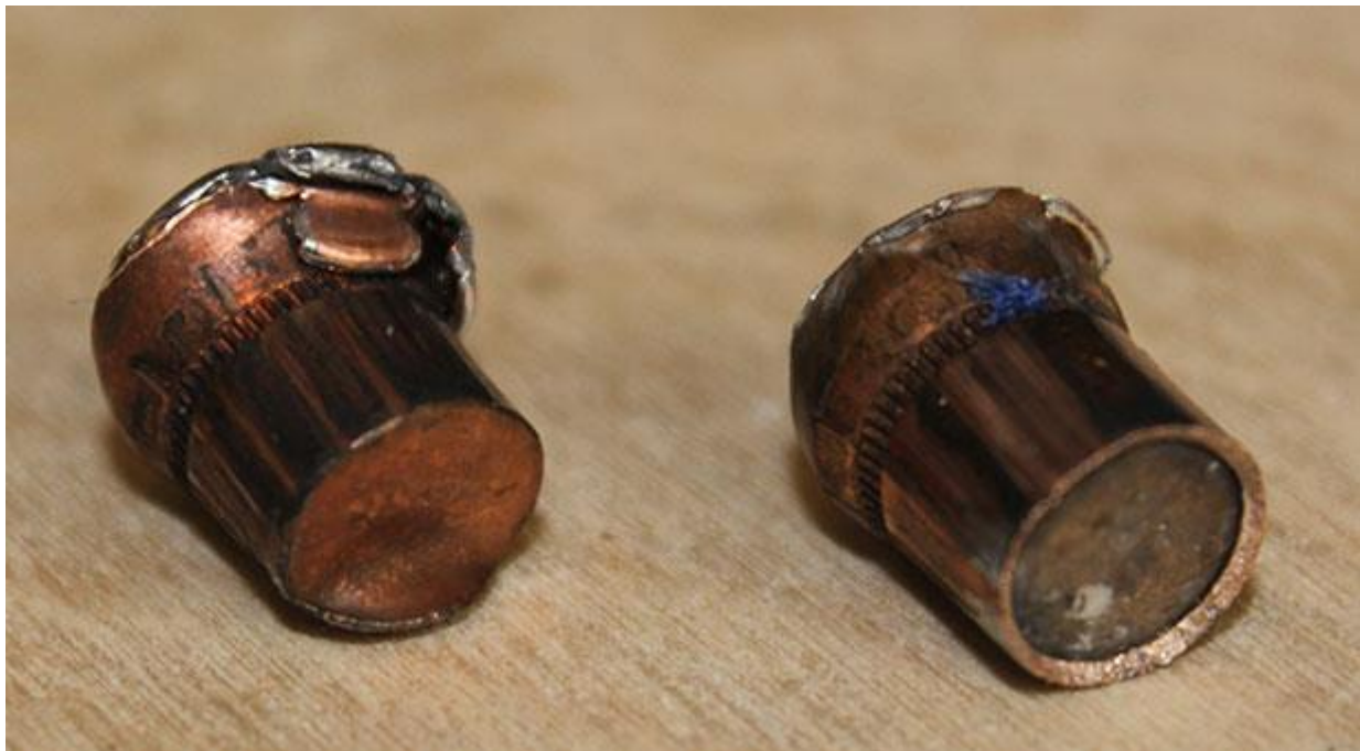
Figure 78: Base View of Bullets Shot through Steel, (Left) Lead Bullet, (Right) Bismuth Bullet
