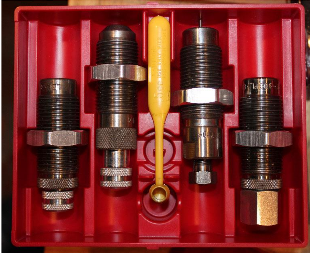
Figure 21: (Left to Right) Crimping Die, Seating Die, Yellow Gunpowder Scoop, Sizing Die, Expander Die
