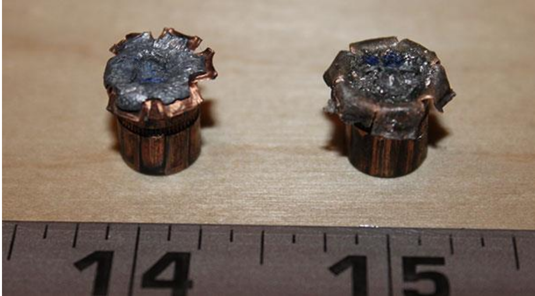
Figure 61: Top View of Bullets Shot through Gypsum Board, (Left) Lead Bullet, (Right) Bismuth Bullet
