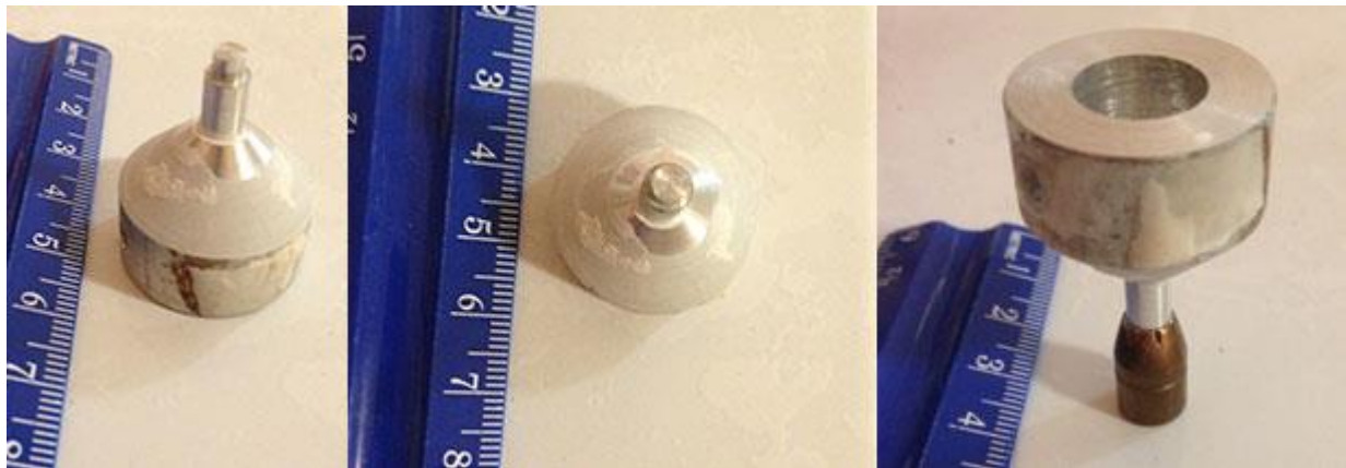
Figure 12: Ruler Measures Centimeters, (Left) Cone Casting Tool, (Middle) Top View of Cone Tool, (Right) Cone Tool Resting on Copper Jacket
